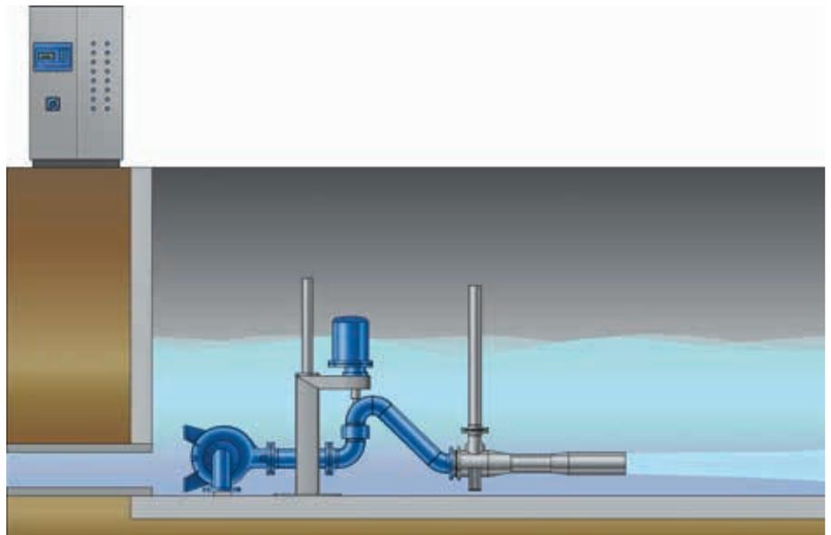
During drainage the sludge is carried out of the system at an even rate to prevent peak demand periods for biological waste water purification.
